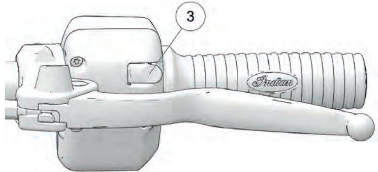
There are trigger switches located on the reverse side of both the right and left ③ switch cubes.
