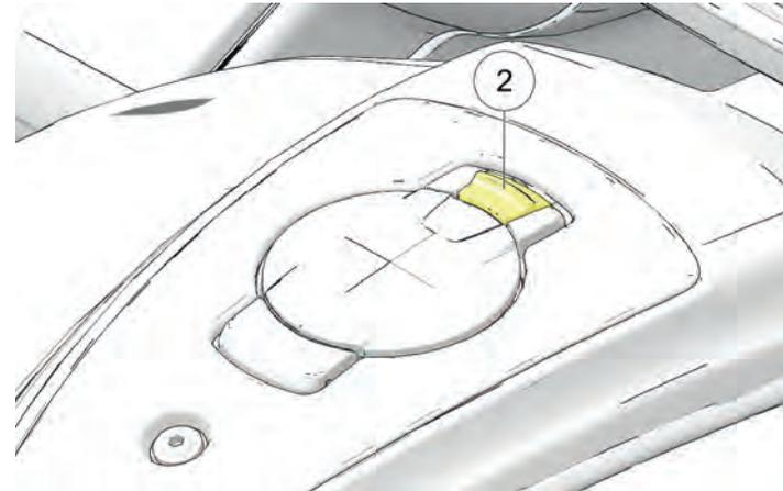
3. Insert the fuel nozzle into the fuel tank filler neck.
