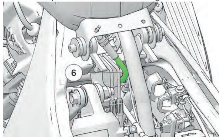
11. On models equipped with an EVAP system, remove the EVAP vent line located above the EVAP canister on the right hand side of the fuel tank ⑦.
