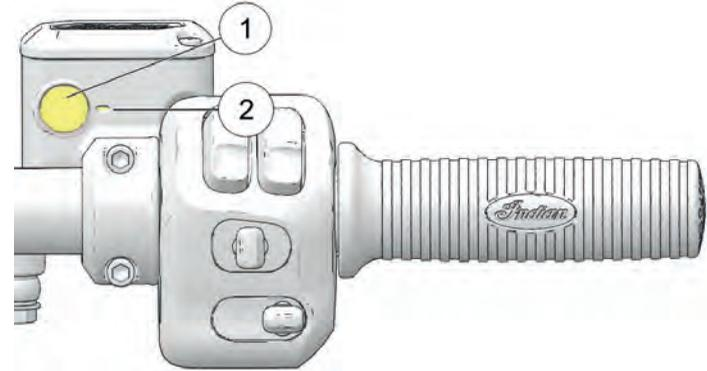
5. Reinstall the diaphragm, cover and screws.
