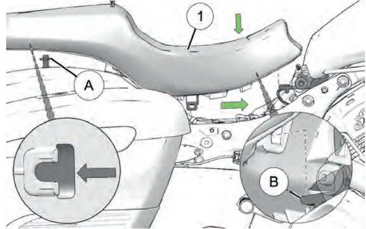
2. Pull straight up on front of seat to ensure a secure fitting.
