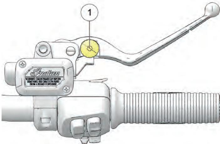
The front brake lever reach (distance to the hand grip) is adjustable. To adjust the front brake lever reach, do the following:
