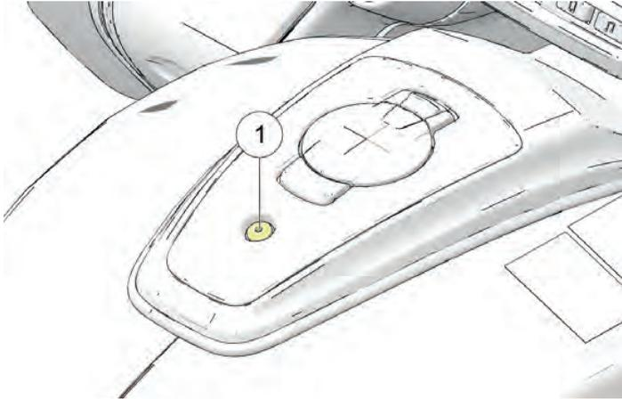
2. With fastener removed, lift the rear of console enough to clear fuel cap and push forward to release front mount from keyway.
