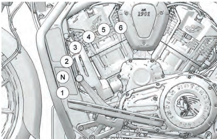
This motorcycle is equipped with a six-speed transmission. Neutral is located between first and second gear.
