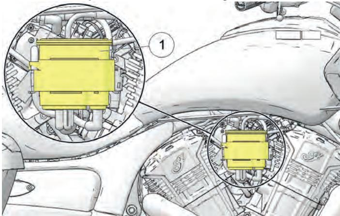
3. Inspect connections at the evaporative emissions canister to be sure they are secure. The vent line coming from the tank should be connected to the port marked "TANK," the purge line should be connected to the port marked "PURGE," and the Atmospheric vent line should be connected to the port marked "AIR."
