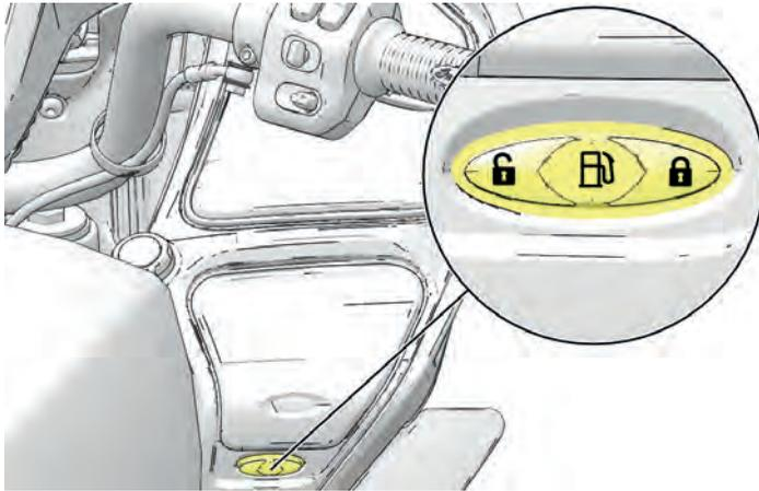
2. Press the fuel cap release button ② (previous page) to release spring loaded cap.
