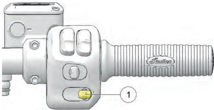
Press up on the switch to adjust the windshield upward. Press down on the switch to adjust the windshield downward. Double tap up or down on the switch to auto-adjust the windshield all the way up or down. If the windshield is traveling and the opposite direction is briefly pressed, the auto travel is canceled.
