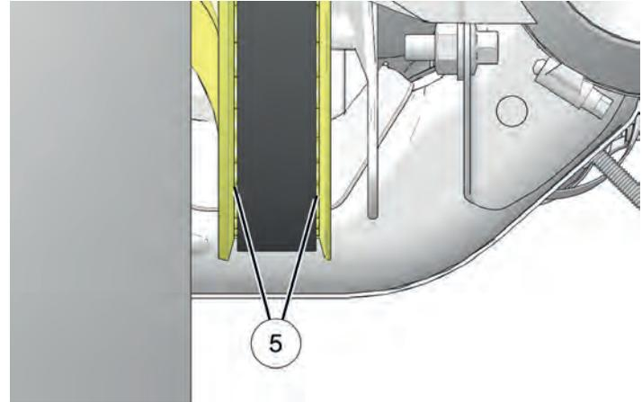
3. If necessary, loosen the axle nut and LEFT SIDE adjuster until belt just moves off the right flange and begins to track down the center of the driven sprocket flange during forward wheel rotation.
