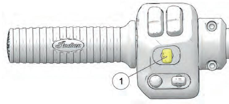
To activate the hazard switch, press on the center of the turn signal switch ①.
