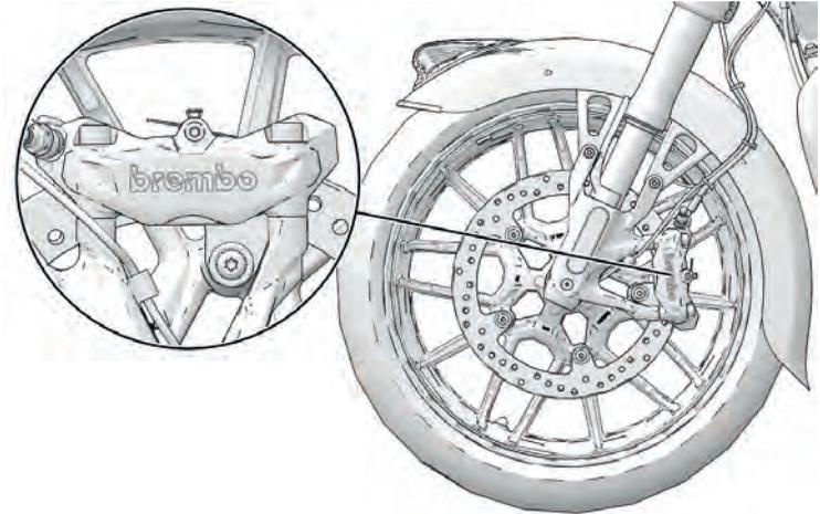
Inspect each front brake pad on both sides of the front discs. Inspect each rear brake pad on both sides of the rear disc. Replace brake pads when the thinnest point of the friction material ② has worn to 1.0 mm. Please see your dealer for this service.
