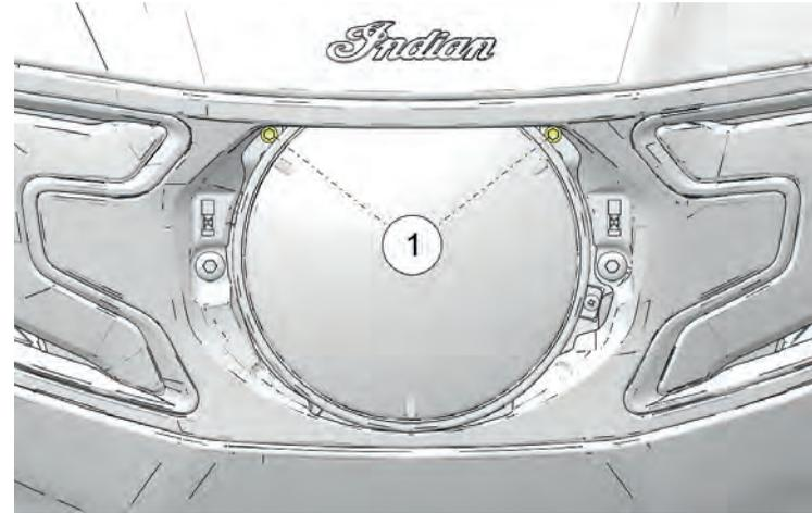
The headlamp adjustment screws ① are located inside the headlamp housing.
