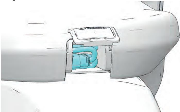
6. Place the cover over the compartment to close the compartment.
