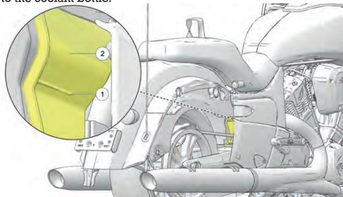
3. Ensure coolant level is above the minimum line ① and below the frame strut ②.
