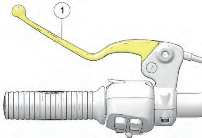
2. Freeplay (gap) is the amount of lever movement from the rest position to the point of cable resistance. Clutch lever freeplay should be 0.5-1.5 mm. Measure the gap between the clutch lever and the lever housing. Adjust clutch lever freeplay if necessary.
