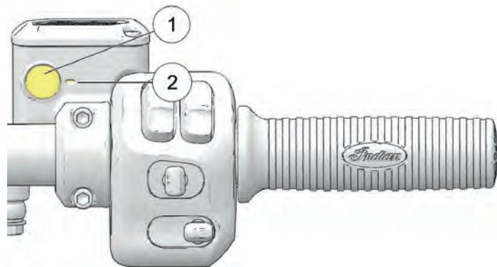
3. The fluid level should be above the minimum indicator mark ② in the sight glass.
