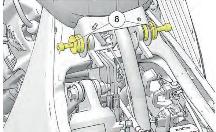
13. Lift rear of tank upward and pull rearward to remove. Place the fuel tank in a secure location with a drain pan to catch any fuel that may leak or drip from disconnected hoses or fittings.
