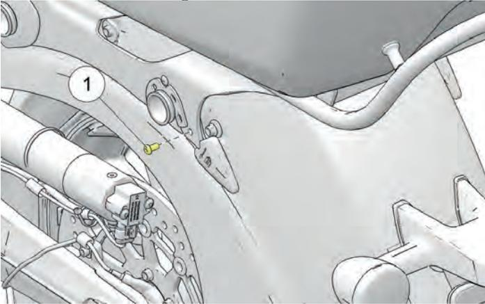
2. Disconnect the antenna harness plugs and trunk harness multi-plug ③.
