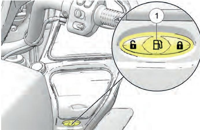
2. Press the full cap release button ② to access the fuel tank.
