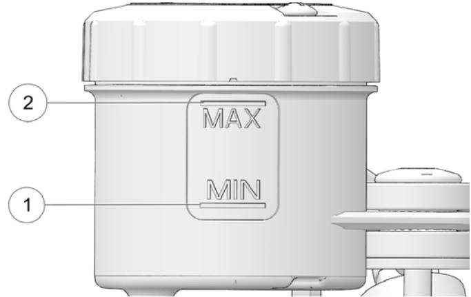
2. View front brake fluid level through the fluid reservoir. The fluid should be clear and between the MIN ① and MAX ② markings. If the fluid level is low, inspect brake pads as outlined on page 126. If pads are not worn beyond the service limit, inspect the brake system for leaks.
