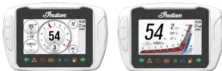
The gauge screen displays the vehicle's speed, current gear, fuel level and range, ambient and engine temperature, odometer, trip meter, and compass. You have two different gauge styles to choose from, round or linear (both shown above). The display style can be changed by swiping up or down on the touchscreen, or by pressing up or down on the select joystick.
