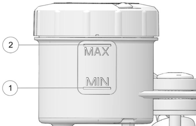
2. View front brake fluid level through the fluid reservoir. The fluid should be clear and between the MIN ① and MAX ② markings.
