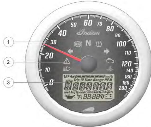
The instrument cluster includes the speedometer, indicator lamps and multi-function display (MFD).
