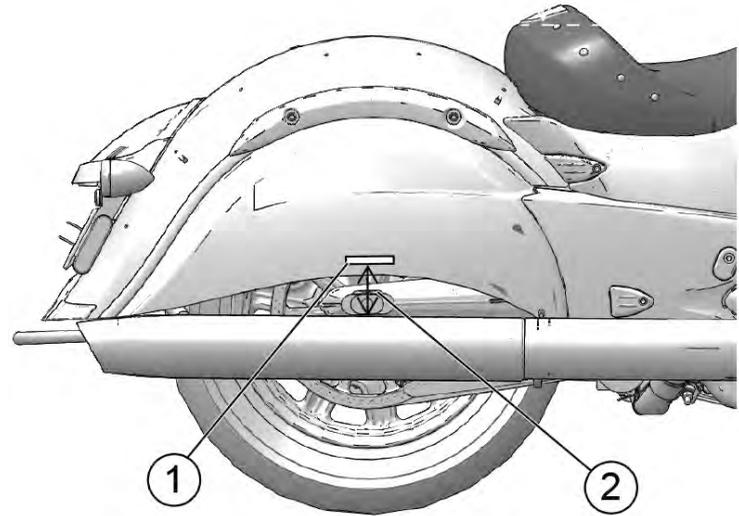
Periodically inspect rear shock preload. For the most comfortable ride and proper ground clearance, adjust preload if ride height is out of specification.
