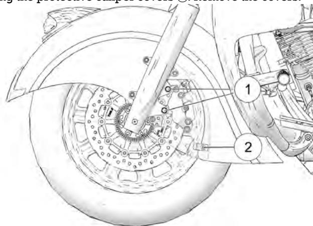
2. Use an inspection mirror, positioned at the front side of the caliper, to view the friction material.
