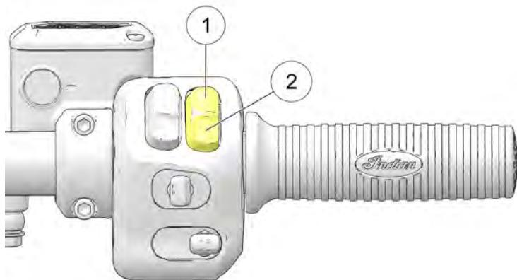
Press the top of the switch (STOP) ① to interrupt the circuits and stop the engine. The engine should not start or run when the switch is in the STOP position.
