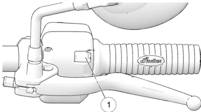
The power switch must be ON for the toggle switches to function. Use the right-hand switch to navigate through menus or accept dialog boxes on the Ride Command display. Use the left-hand switch to back out of menus, decline dialog boxes, hang up phone calls, and toggle through display screens.
