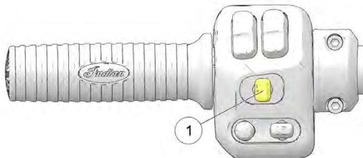
To activate the hazard switch, press on the center of the turn signal switch ①.
