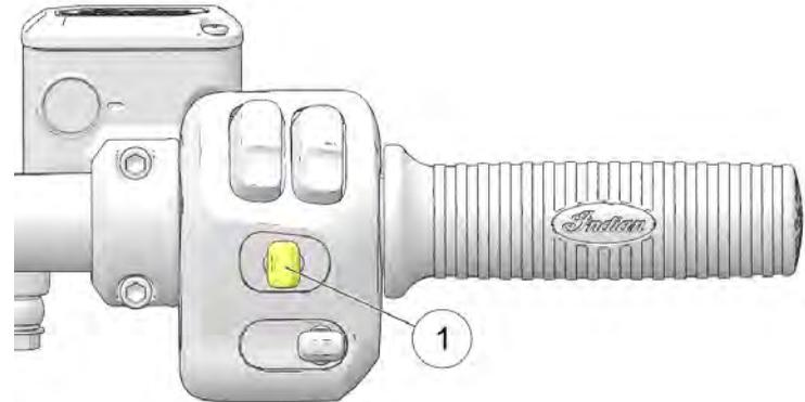
Cruise control can be activated and adjusted from the right control using the Cruise Control Switch ①.
