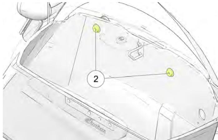
6. Tilt the saddlebag away from the frame of the vehicle to remove it.
