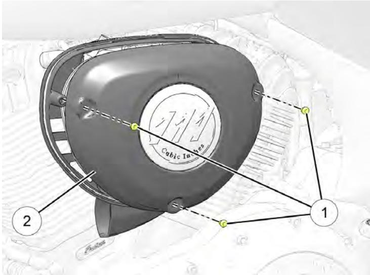
1. Remove the air box cover screws ①, and remove the cover ②.
