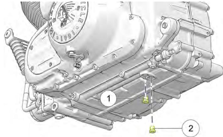
4. Remove the drain plugs. Allow the oil to drain completely.
