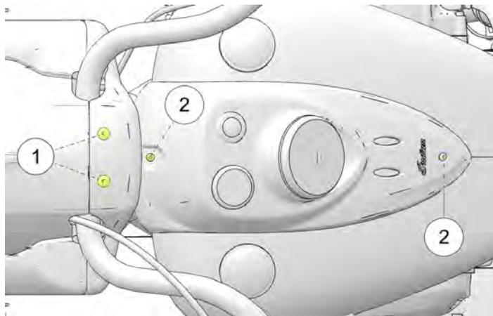
3. Remove two fasteners ② securing the console cover to the fuel tank and lift console back and set on protected fuel tank.
