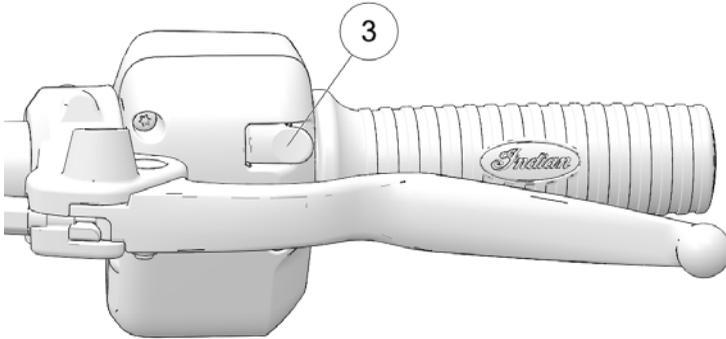
There are trigger switches located on the reverse side of both the right and left ③ switch cubes.
