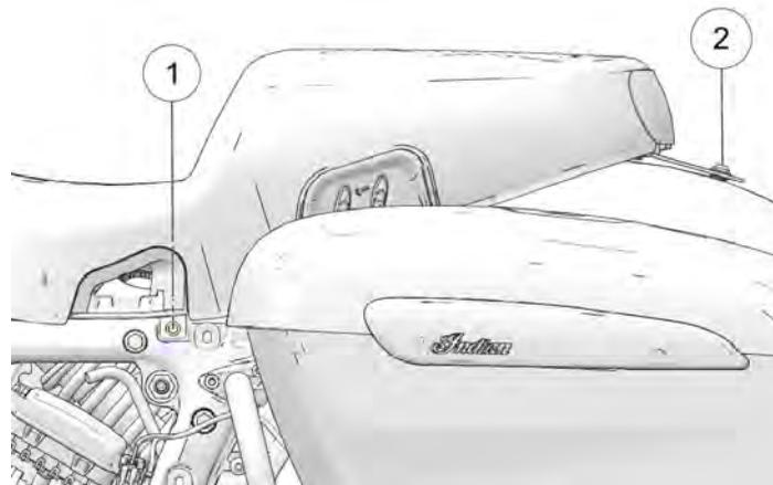
6. Remove the rear bracket bolt ②, washer and nylon grommet from the passenger portion of the seat.
