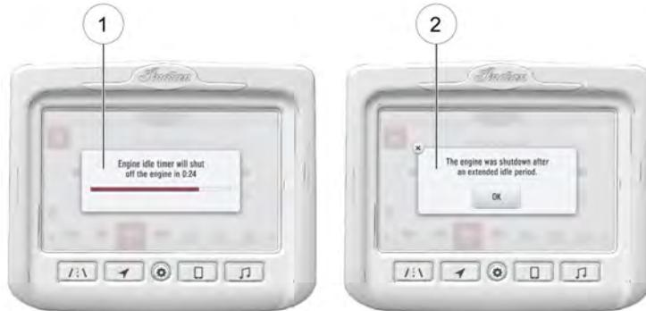
For motorcycles equipped with Ride Command, a notification will display a countdown timer to warn that the engine is about to shut off ①. After the time has elapsed and the engine is shut off, a subsequent notification will be displayed ②. After the engine shuts off, the engine can re-started by pressing the starter switch.
