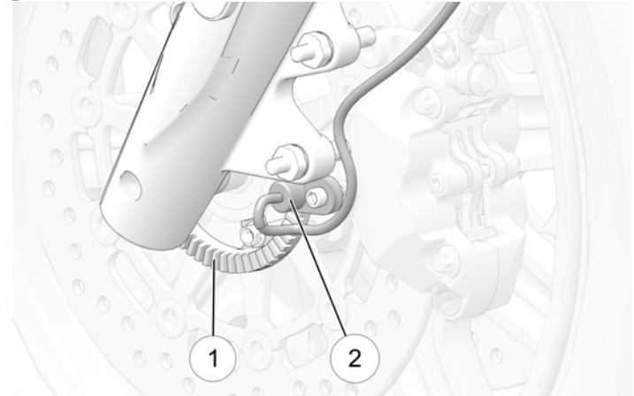
2. Inspect for debris adhering to the end of the wheel speed sensors ②. If contamination is observed, or if you are unable to visually inspect, slide a thin towel across the face of the sensor between the sensor and the tone ring to remove any potential debris.
