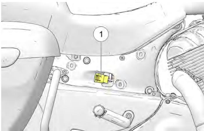
3. Disconnect the saddlebag lock wiring near the seat ①.
