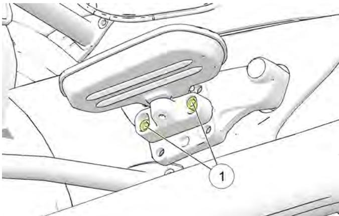
To adjust the height, remove both attachment screws. Move the floorboard assembly to the next hole position, then reinstall the fasteners, adjust the angle and tighten the fasteners.
