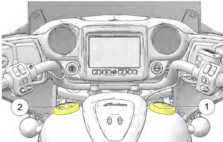
Turn the fuel cap counter-clockwise to remove it. If the fuel cap is equipped with a tether, carefully rest fuel cap on the tank so that the rubber bumper is contacting the tank. See page 72 for fueling instructions. To tighten the cap, turn it clockwise until the seal compresses onto the tank, then continue to tighten until the cap ratchets several times.
