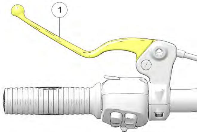
2. Freeplay (gap) is the amount of lever movement from the rest position to the point of cable resistance. Clutch lever freeplay should be 0.5-1.5 mm. Measure the gap between the clutch lever and the lever housing. See page 120. Adjust clutch lever freeplay if necessary.
