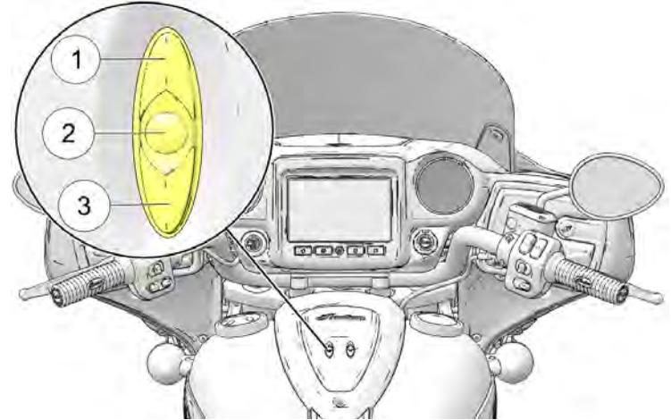
The heaters have 10 heat levels, ranging from OFF (level 0) to highest heat (level 10). Press and release the top of the switch ① to increase the heat level by one increment. Press and release the bottom of the switch ③ to decrease heat by one increment.
