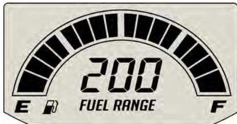
The fuel gauge displays fuel level. For the most accurate reading, sit on the motorcycle and bring it to the upright position.
