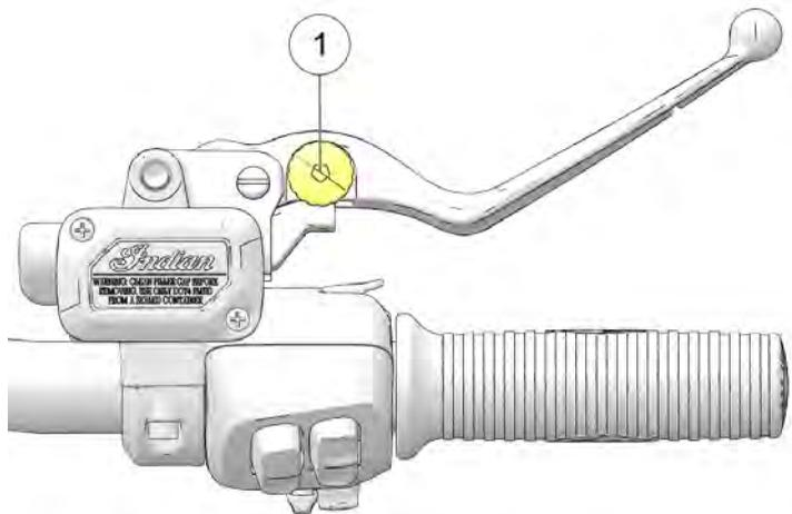
The front brake lever reach (distance to the hand grip) is adjustable. To adjust the front brake lever reach, do the following:
