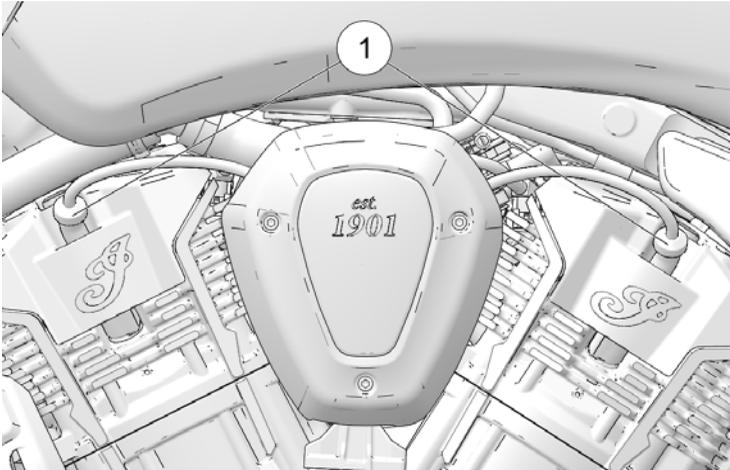
3. Pull upward on the spark plug boots (not the wires) to remove the boots.
