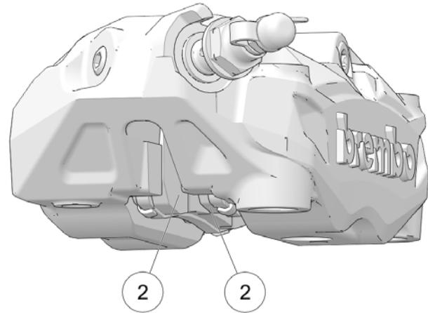
Inspect each front brake pad on both sides of the front disc. Inspect each rear brake pad on both sides of the rear disc. Replace brake pads when the thinnest point of the friction material ② has worn to 1.0 mm. Please see your dealer for this service.
