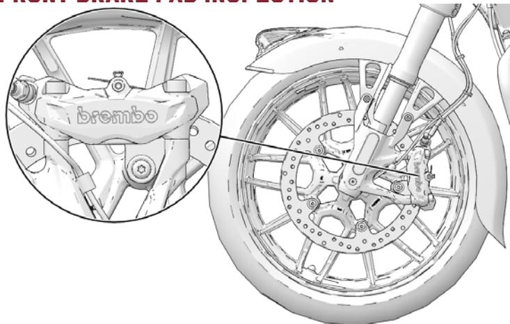
1. Position the motorcycle on the sidestand with the handlebars turned to the left.
