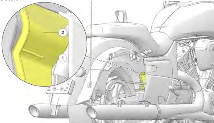
3. With the motorcycle vertical (not on the side stand), ensure coolant level is above the minimum line ① and below the frame strut ②.
