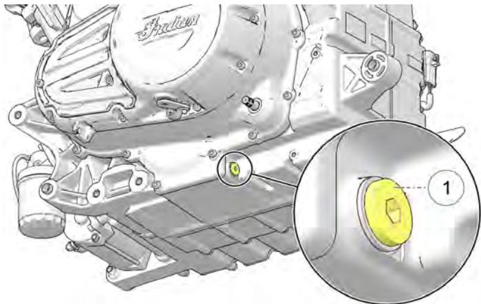
4. Remove the drain plug. Allow the oil to drain completely.
