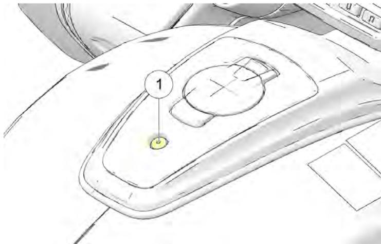
1. Ensure engine is not running before attempting to manually unlock fuel cap
