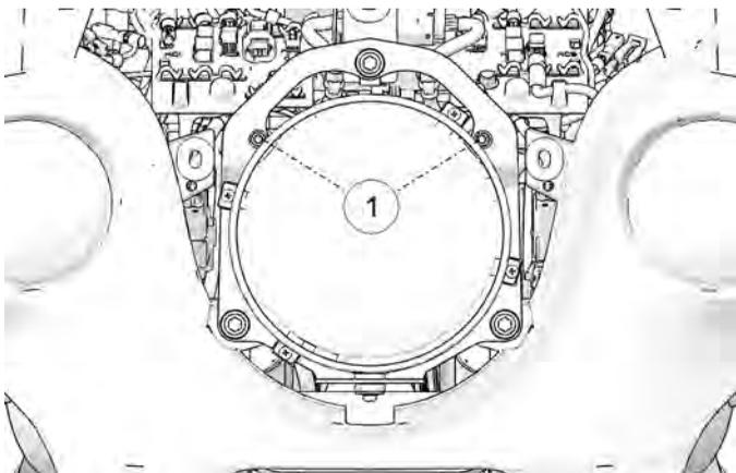
1. Remove the two headlight bezel screws (*fairing models only*) and remove the bezel from the fairing. Reinstall the bezel after adjusting the headlamp.
