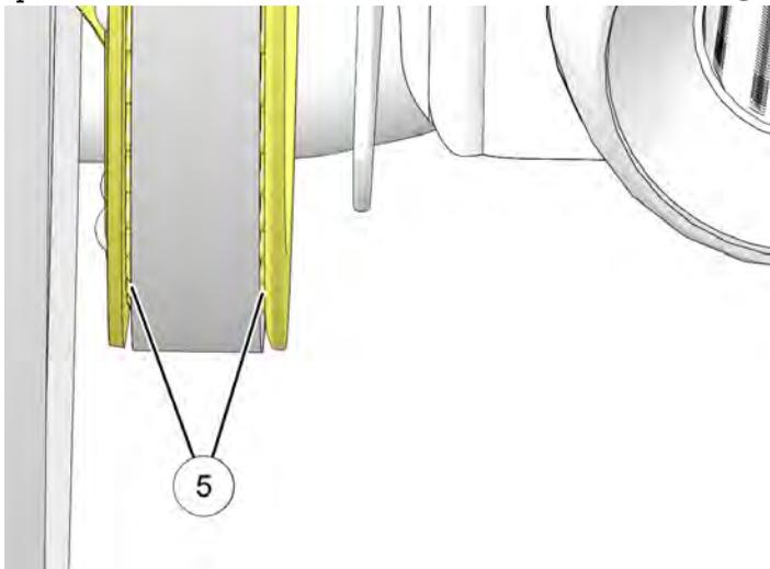
3. If necessary, loosen the axle nut and LEFT SIDE adjuster until belt just moves off the right flange and begins to track down the center of the driven sprocket flange during forward wheel rotation.
