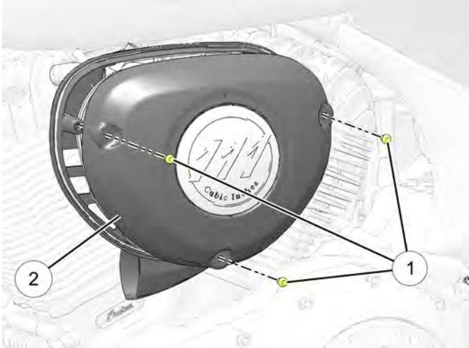
2. Remove the three air filter screws ③ and remove the air filter assembly.
