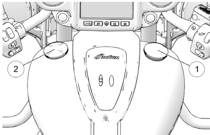
1. Turn the fuel cap counter-clockwise to remove it.
