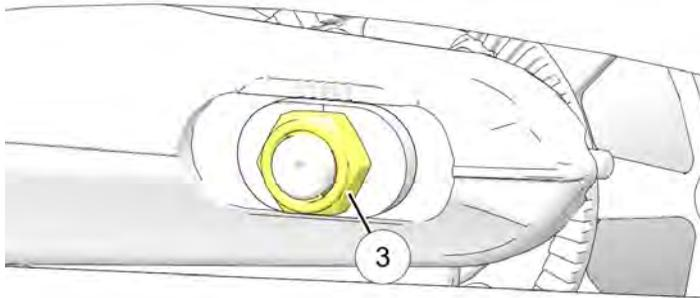
5. Turn the RIGHT SIDE adjuster nut ④ to achieve proper belt tension.
