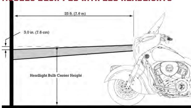
With the headlight switched to LOW beam, the top of the highest intensity (appears as a diamond shape) should be 3.0 in (7.6 cm) below the height of the headlight bulb when centered straight ahead at 25 feet (7.62 m).
