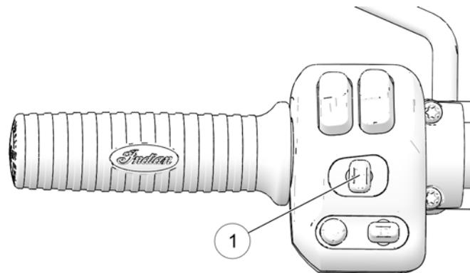
To activate the hazard switch, press on the center of the turn signal switch ①.
