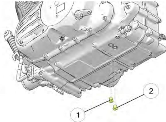
4. Remove the drain plugs. Allow the oil to drain completely.
