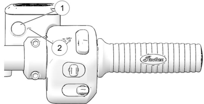
3. The fluid level should be above the minimum indicator mark ② in the sight glass.
