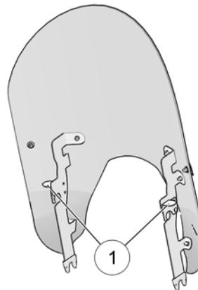
2. From the front of the motorcycle, pull firmly on the upper windshield to remove the windshield from the upper mounts, then pull the windshield upward and away from motorcycle.
