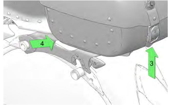
3. Lift up on the rear of the trunk ③ and slide rearward ④ to release the trunk from the motorcycle.
