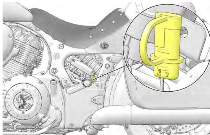
1. Following the charger manufacturer's instructions, use a battery charger designed for use with 12-volt batteries. The charger should have a maximum charging rate of 1.8 amps. Charge the battery for approximately 10 hours at a rate of 1.8 amps. If you use a taper or trickle charger, it will take longer to charge the battery.
