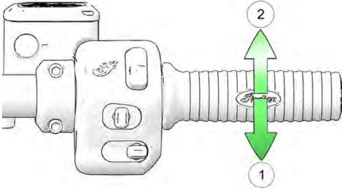
The control grip is spring loaded. When you release the grip, the throttle returns to the idle position.
