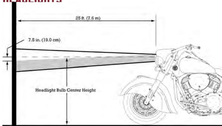
With the headlight switched to HIGH beam, the center of highest intensity (appears as a diamond shape) should be 7.5 in (19 cm) below the height of the headlight bulb when centered straight ahead at 25 feet (7.62 m).
