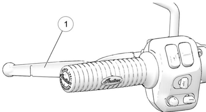
2. Freeplay (gap) is the amount of lever movement from the rest position to the point of cable resistance. Clutch lever freeplay should be 0.5-1.5 mm. Measure the gap between the clutch lever and the lever housing. See page 122. Adjust clutch lever freeplay if necessary.
