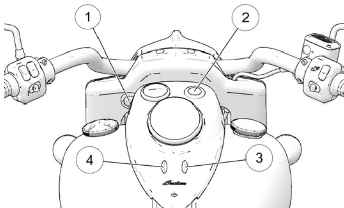
① Auxiliary Light Switch (if equipped)
