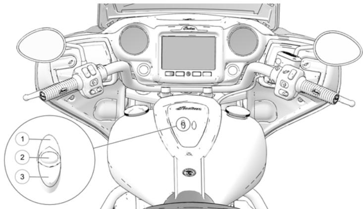
The heaters have 10 heat levels, ranging from OFF (level 0) to highest heat (level 10). Press and release the top of the switch ① to increase the heat level by one increment. Press and release the bottom of the switch ③ to decrease heat by one increment.
