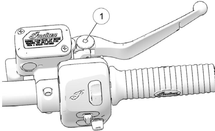
1. Gently push and hold the lever away from the hand grip. The adjuster wheel ① is located on top of the lever.
